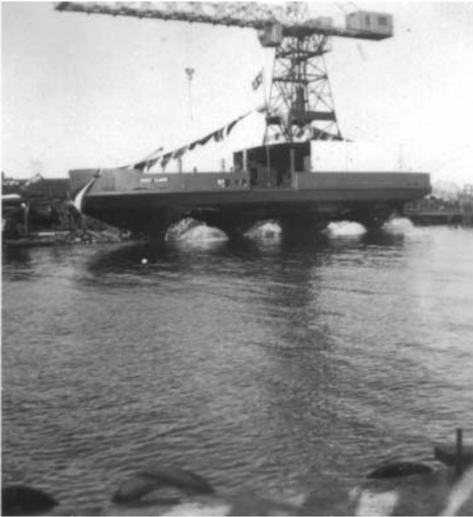
The MV Amherst Islander (1955) being side-launched in Kingstons Shipyards (above), and afloat (below) (despite a few missing welds in the hull plating ). Photos by Garnet McDonald
